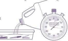
Rinse tools with water and leave to dry or dry manually using clean, lint-free cloth\*\*
